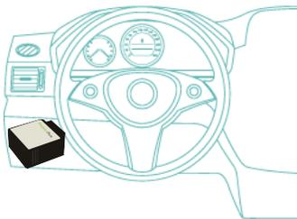
Hold the unit in place and mark the location for the velcro. Attach one side of the velcro to the back of the unit and one to the dash where the unit is going.
